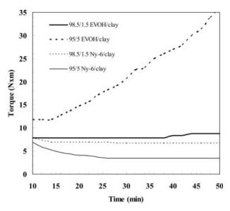
Figure 9. Brabender plastograms of near 98.5/1.5 and 95/5 Ny-6/clay and 98.5/1.5 and 95/5 EVOH/clay, at 250  $^\circ$ C and 20 rpm.<sup>14</sup>
