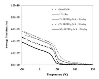
**Figure 7.** Storage modulus of EVOH/clay systems containing LLDPE-*g*-MA.<sup>11</sup>
