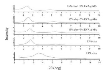
Figure 5. X-ray diffraction patterns of EVOH/clay systems containing EVA-g-MA.<sup>11</sup>
