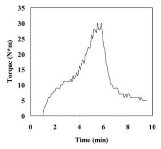
Figure 2. Haake plastogram of an 85/15 EVOH/ treated clay blend at 230  $^{\circ}\mathrm{C}$  and 150 rpm.  $^{9}$
