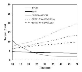
Figure 8. Brabender plastograms of neat EVOH, Ny-6, 50/50 Ny-6/EVOH, 50/50/1.5 and 50/50/5 Ny-6/EVOH/clay, at 250  $^{\circ}$ C and 20 rpm.<sup>14</sup>
