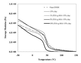
**Figure 6.** Storage modulus of EVOH/clay systems containing EVA-g-MA.<sup>11</sup>
