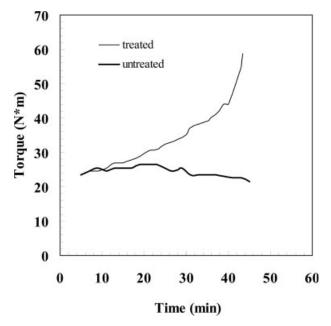
**Figure 1.** Brabender plastograms of 85/15 EOH/clay blends at 230  $^{\circ}$ C and 60 rpm.<sup>9</sup>
