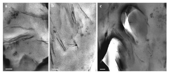
**Figure 12.** TEM micrographs of 50/50/1.5 Ny-6/EVOH/clay Brabender cell mixing at 250 °C for 50 min (bar = nm).<sup>14</sup>
