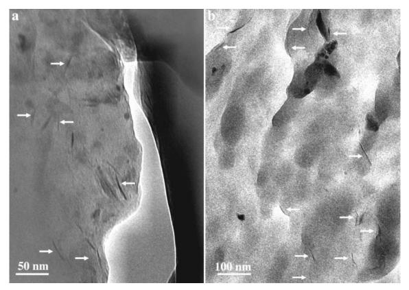
**Figure 14.** TEM micrographs of 99/1 EVOH/clay composite after first extrusion pass at 200  $^{\circ}$ C and 40 rpm, and injection molding at 200  $^{\circ}$ C.<sup>14</sup>
