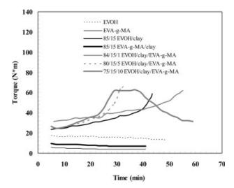
**Figure 4.** Brabender plastograms of EVOH/clay systems containing EVA-g-MA, at 230 °C and 60 rpm.<sup>11</sup>
