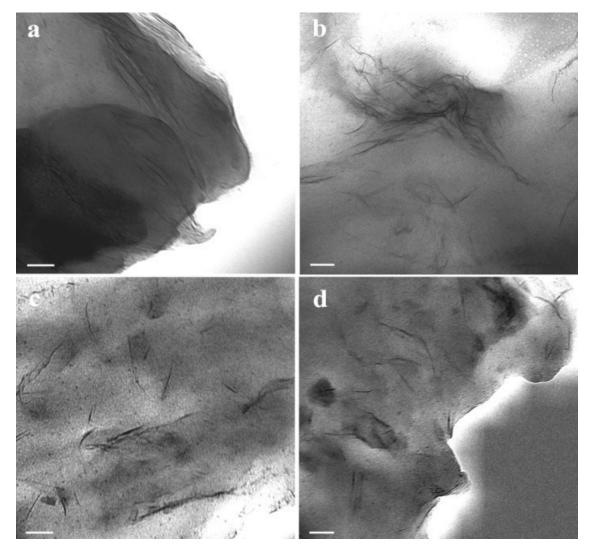
Figure 11. TEM micrographs of 50/50/5 Ny-6/EVOH/clay Brabender cell mixing, at 250  $^{\circ}$ C for 50 min (bar = 50 min).<sup>14</sup>
