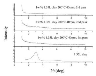
**Figure 13.** X-ray diffraction patterns of 99/1 EVOH/ 1.35L clay composite after first, second, and third extrusion passes at 200  $^{\circ}$ C and 40 rpm, and injection molding at 200  $^{\circ}$ C.<sup>14</sup>
