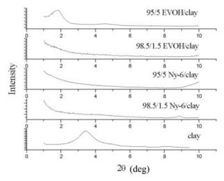
**Figure 10.** X-ray diffraction patterns of neat clay, 98.5/1.5 and 95/5 Ny-6/clay and 98.5/1.5 and 95/5 EVOH/ clay Brabender cell mixing, at 250  $^{\circ}$ C for 50 min.<sup>14</sup>
